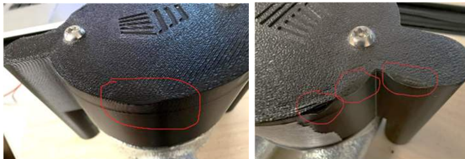
Figure 5 Superficial damage slight indentations to the HSJB housing
